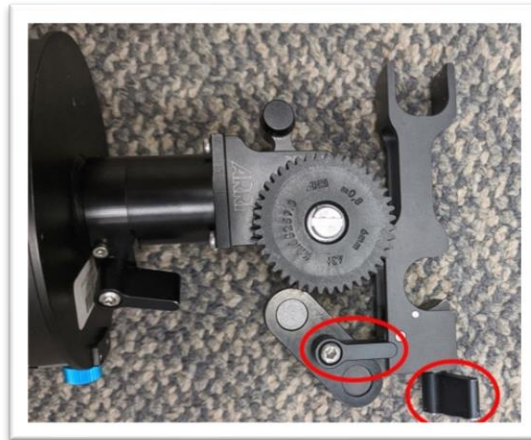
The follow focus attachment screws are indicated by red circles in this photo.
