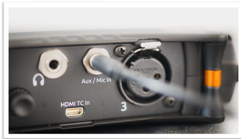
Connecting the Tentacle to the MixPre-3 or 6 via the Aux/Mic In jack.
